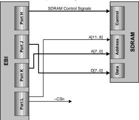
If SRAM and SRAM LPC is used together with SDRAM, consider that address lines A16 to A19 are moved to the lower four bits of Port L. This applies to all SRAM and SRAM LPC configurations that share address lines A16 to A19 with the Chip Select lines. Refer to Section 4.1 below for details.
